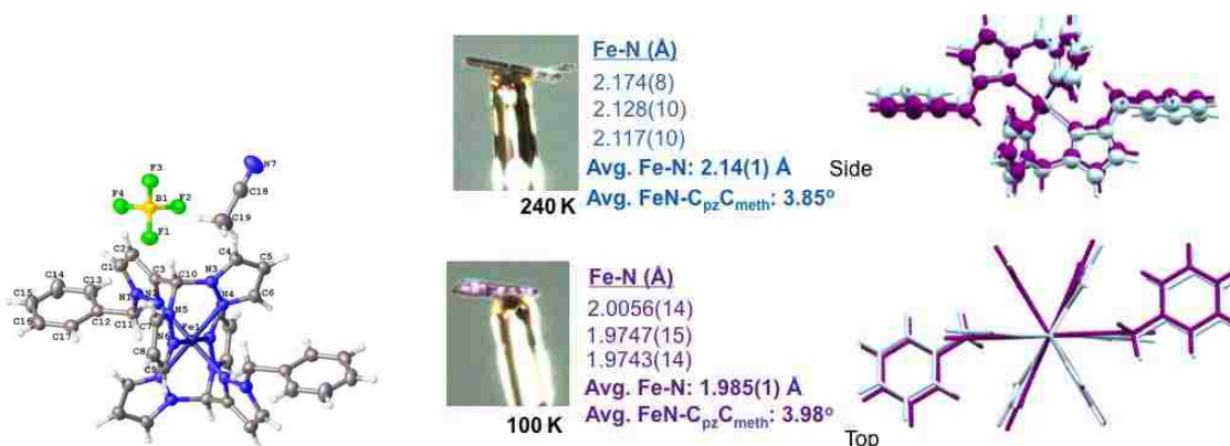
Figure 3.3. Left: View of the structure of (3.1)(\text{BF}_4)_2 \cdot 2\text{CH}_3\text{CN} at 100 K. Center: Photographs of crystals at 240 K and 100 K and list of bond distances and angles. Right: Overlays of dications at high temperature (purple) and low temperature (pale blue).
