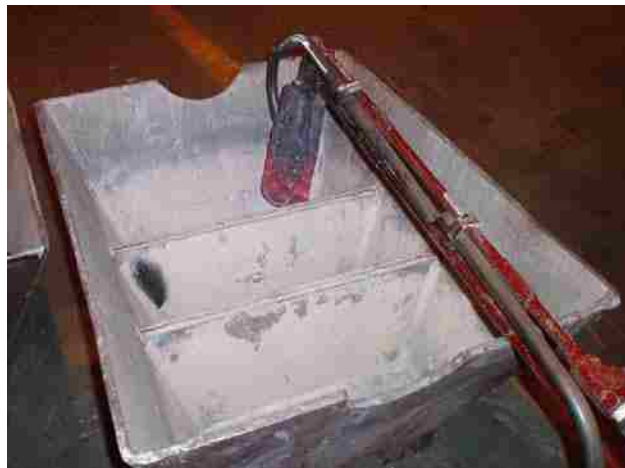
Figure 27. V-Cal preheating operation prior to the secondary ingot manufacture.
