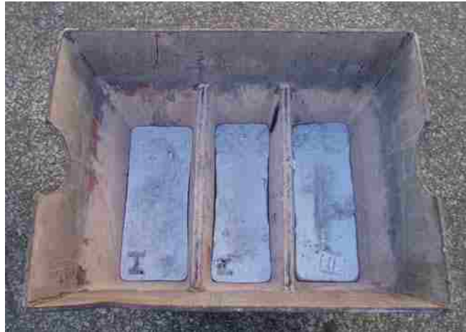
Figure 28. One of the V-Cal castings made indicating three (3) ingots, each with a different MMC target chemistry.
