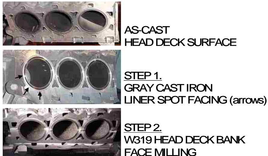
Figure 49. 3.0L V6 sand cast W319 engine block right hand head deck surface indicating the as-cast head deck condition, the liner 'spot facing' operation and the fully face milled 'cubed' head deck condition.
