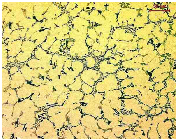
Figure 86. 7.5kW UMSA test sample cross-section at a distance of 15mm from the chilled end indicating the overall microstructural refinement of the as-cast structure due to the MMAC additions.
