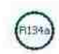
Figure F-1: AMESim icon for sub-model TPF_FP01. This icon is required when running simulations with two-phase materials. This sub-model contains all the refrigerant property data for all of the simulations in the present thesis.
