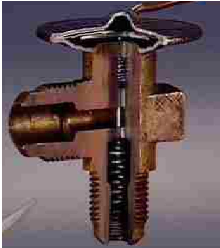
Figure F-13: Cutaway of an actual TXV. The TXV geometry does not correspond directly to Figure F-12, but it serves to compliment the schematic previously shown.
