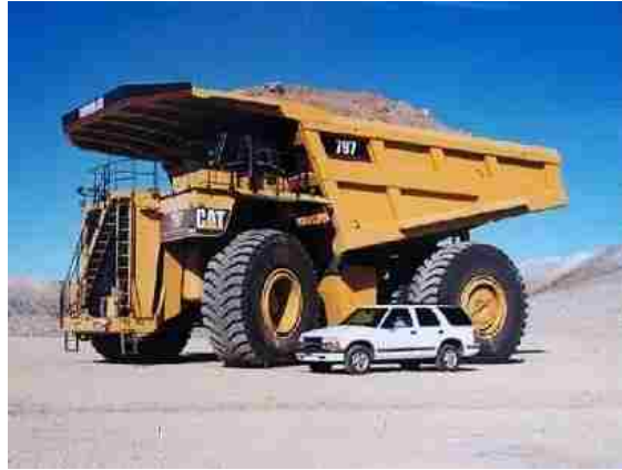
Figure 1.2 The size difference between OTR tires and on-the-road tires [7]. (Reprinted Courtesy of Caterpillar Inc.)
