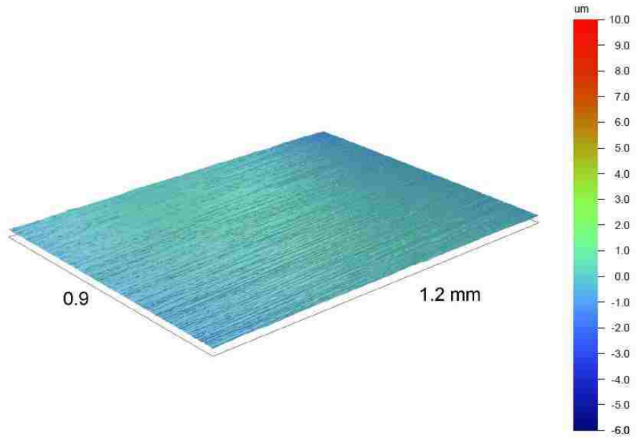
Figure 6-19 Sample G800 3D roughness before corrosion
