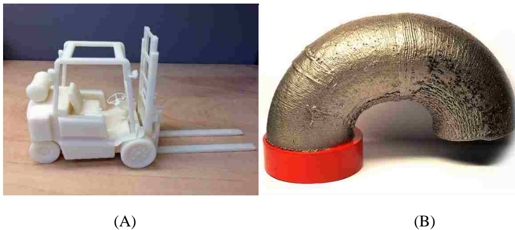
Figure 1: Additive manufacturing prototypes- (A) FDM and (B) laser cladding operations
