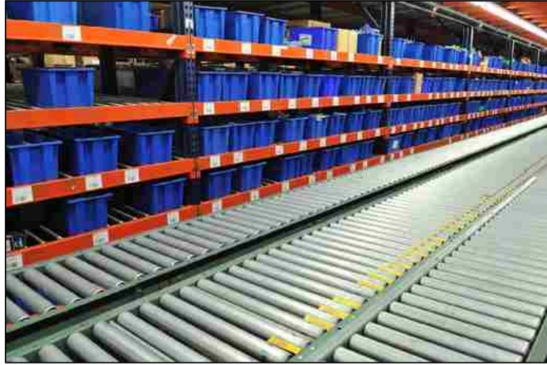
Figure 4.15 – Example of warehouse equipment for standard totes. [24]
