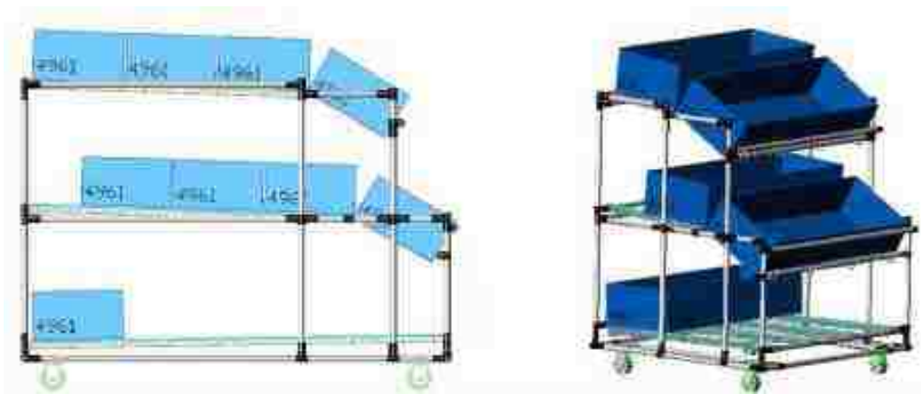
Figure 4.16 – Example of line side equipment for standard totes. [23]
