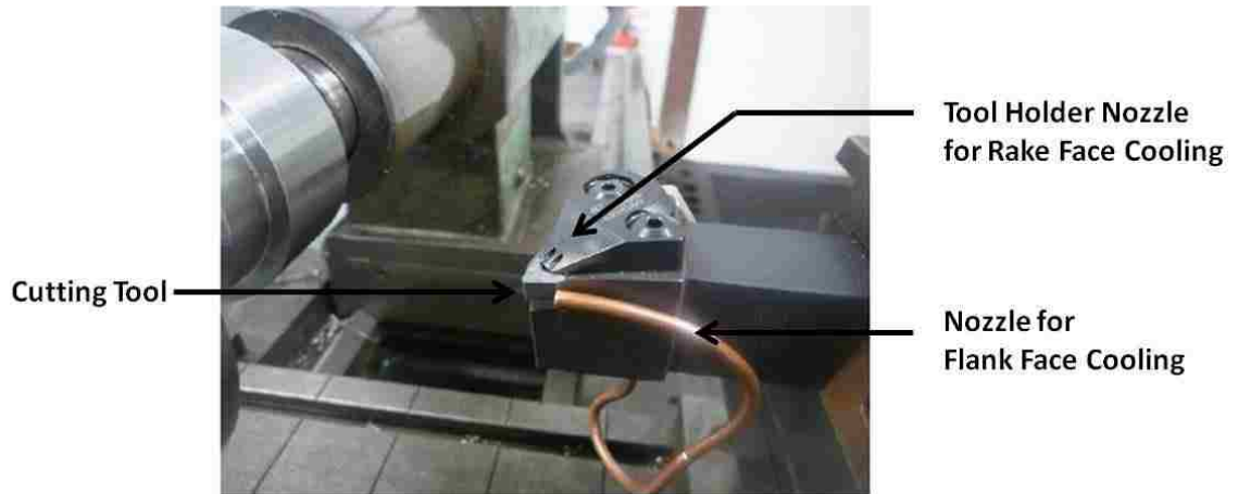
Figure 2.44 Photograph of liquid nitrogen coolant delivery system showing modified tool holder nozzle for rake face cooling with an additional flank face cooling nozzle [85].
