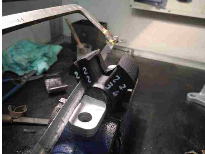
Figure 9: Removal of rubber segments to prepare quasi-static material characterization specimens (simple compression specimen preparation shown).
