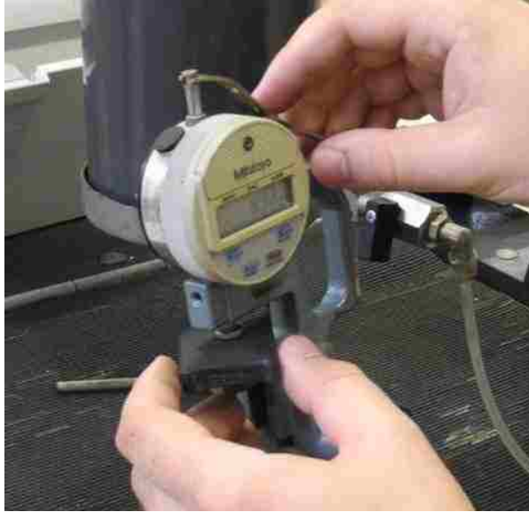
Figure 11: Mitutoyo measuring device consistent with ASTM standard D3767 for measuring thickness of rubber components with a specified force of compression.
