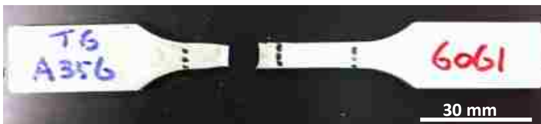
Figure 4-30 Fractured tensile specimen of welded T6 A356/6061 alloys.
