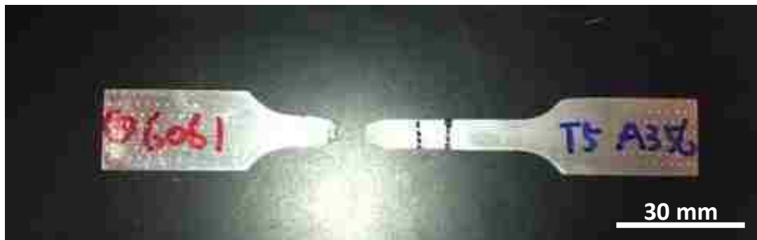
Figure 4-27 Fractured tensile specimen of welded T5 A356/6061 alloys
