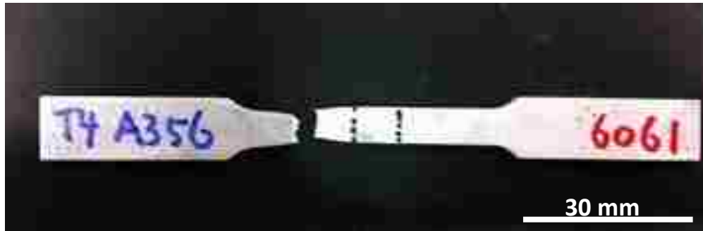
Figure 4-23 Fractured tensile specimen of welded T4 A356/6061 alloys.
