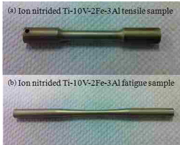
Figure 3.12 Real image shown of (a) the tensile test sample, and (b) fatigue test sample which have been ion nitrided according to optimized nitriding condition selected from Section 3.5.
