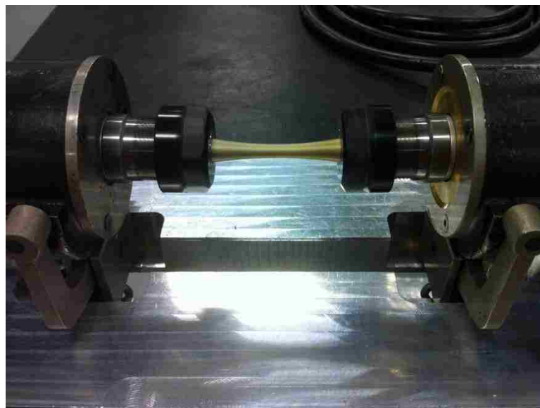
Figure 3.15 Bending rotation fatigue tests ( R = -1 ) are performed on untreated Ti-10V-2Fe-3Al using R.R. Moore type fatigue machine at the 50 Hz in room temperature.
