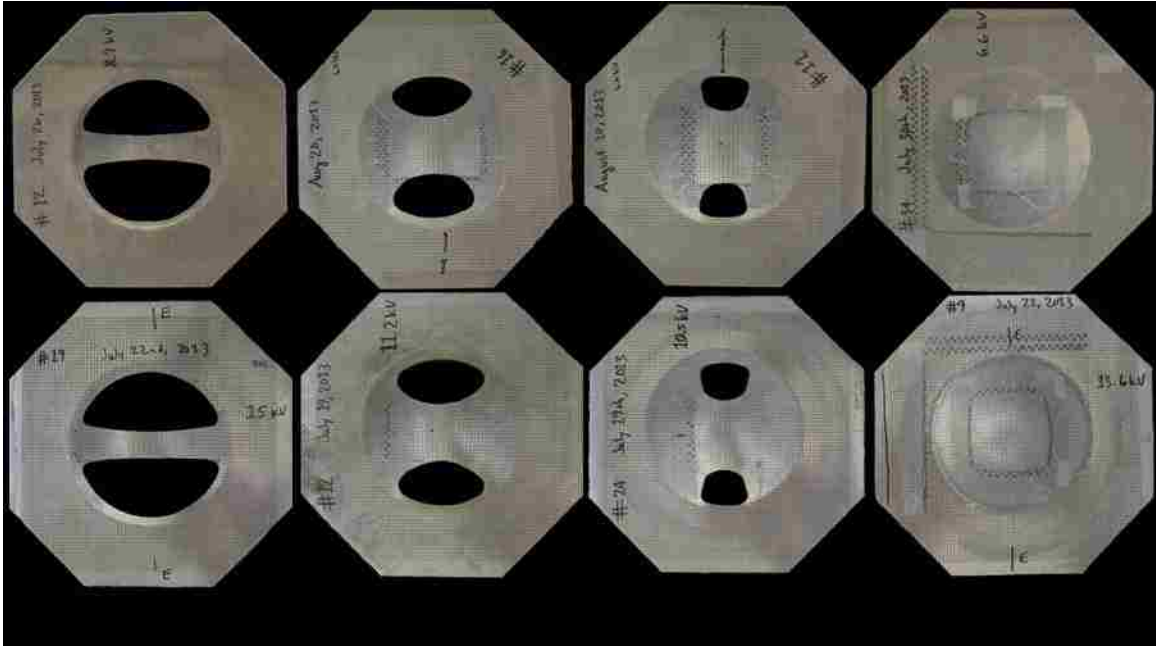
Figure 4-16: Necked specimens in each strain path for AA5182-O (top row) and DP600 (bottom row).
