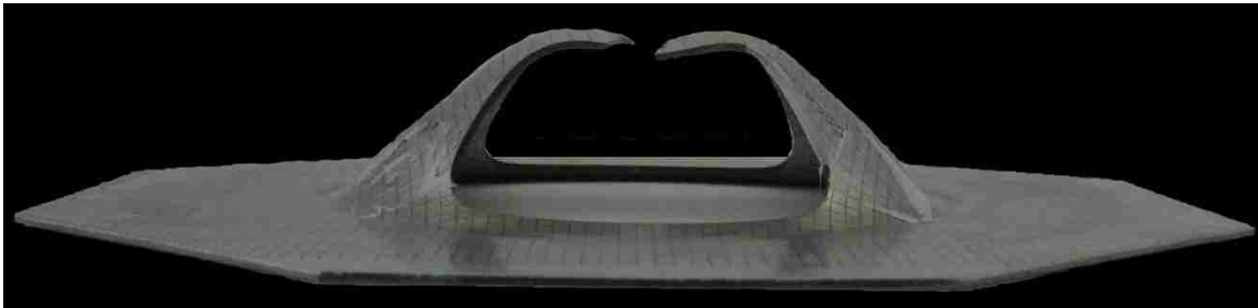
Figure 4-46: Side profile of a mini-die forming specimen with the die higher than the free forming height.
