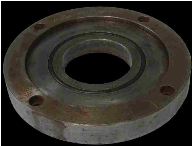
Figure 3-5: The chamber ring that was added to the new chamber to increase the volume.
