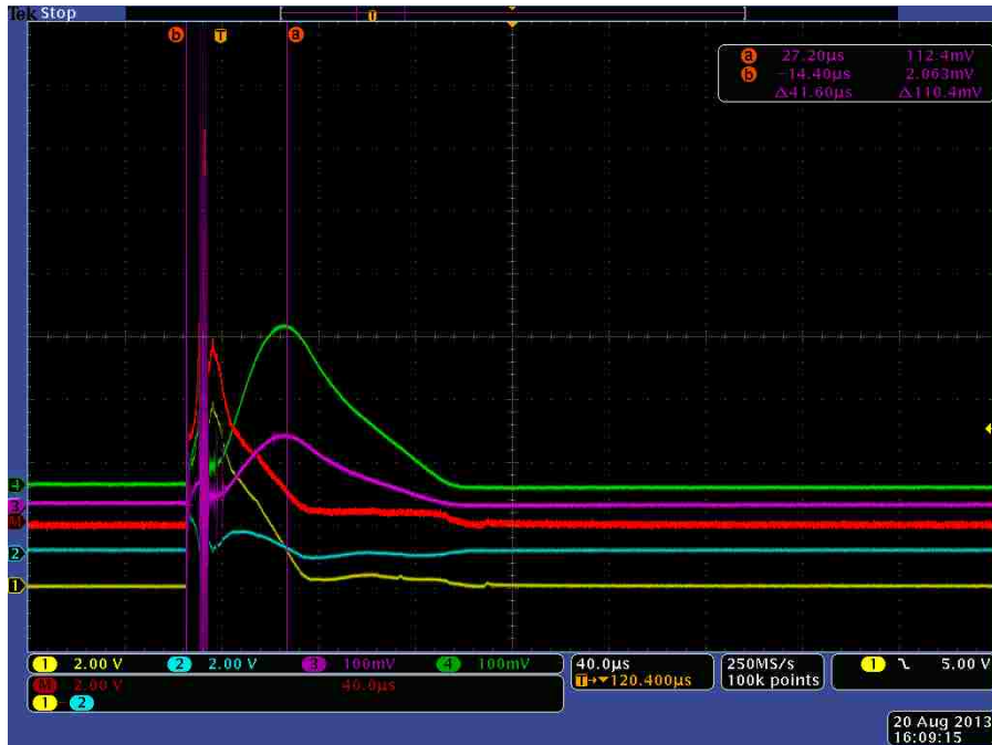
Figure 3-15: Recordings from the oscilloscope for a 6.1kV discharge used to measure positive voltage (1-yellow), negative voltage (2-blue), the differential voltage (M-red), the current at the chamber (3-purple), and the current at the Magnepress (4-green).
