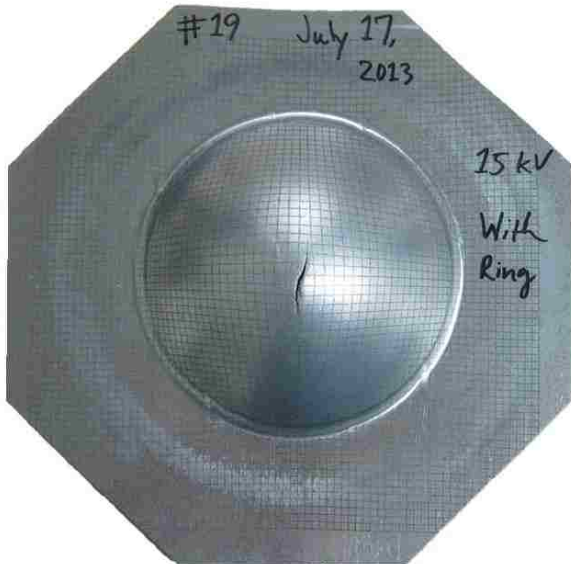
Figure 4-25: Splitting in biaxial DP600 specimens.
