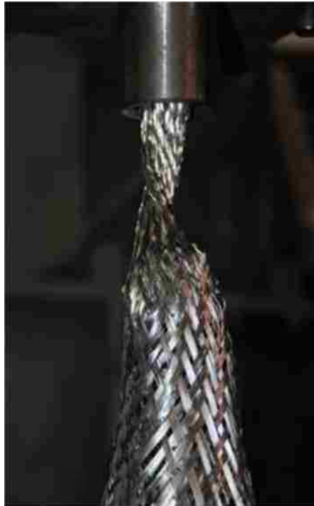
Figure 19: Tapered profile of specimen 2 for low diameter high density circular core tubular assembly prior to failure.
