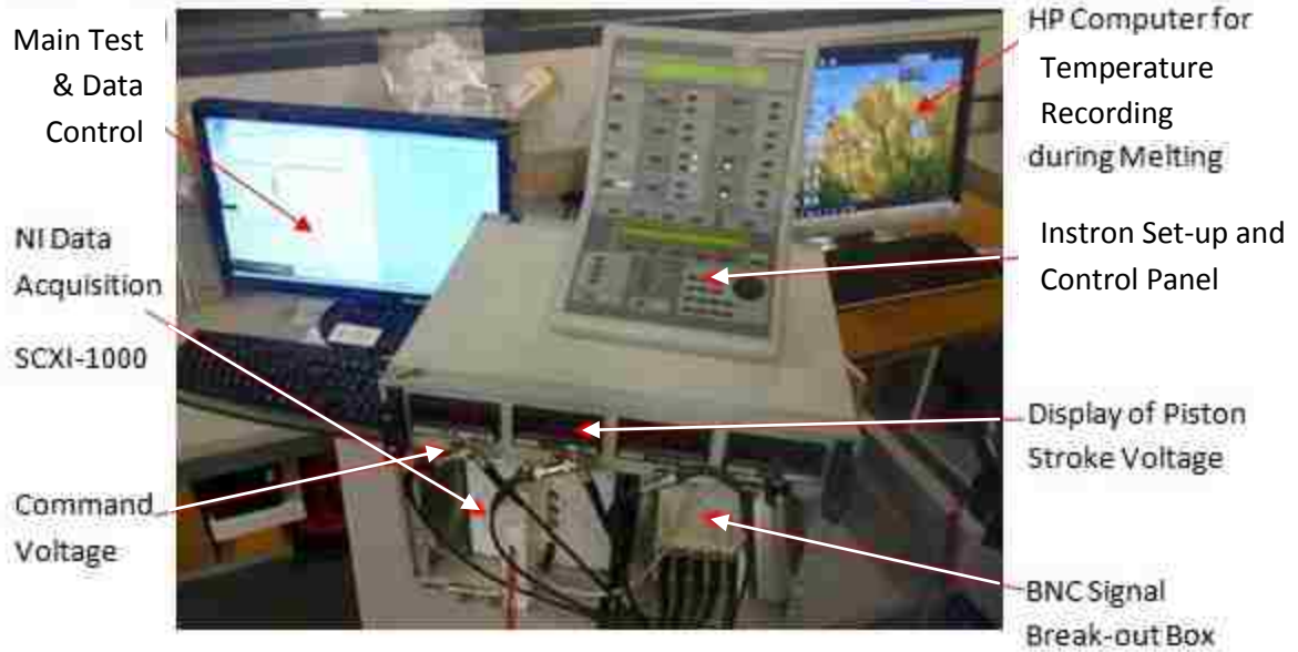
Figure 30 - SC-UMSA test set-up, data recording and data collection devices: main test and data control computer monitor on left, SCXI-1000 at center, and HP system for monitoring temperature of thermocouples at the right.
