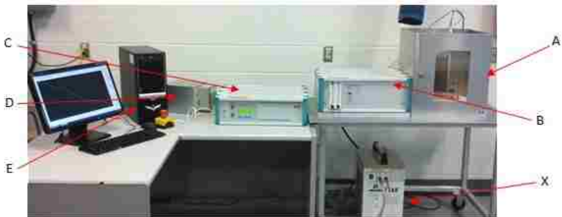
Figure 38 - Photograph of the HT UMSA Technology Platform. A – Melting and environmental chamber, B - heat exchanging systems, C – Power supply, D – Data acquisition system, E –Desktop computer, X – Water cooling pump.
