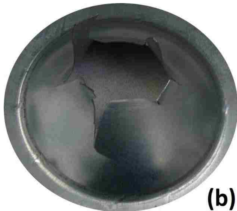
Figure 5-5 (a) DP500 and (b) DP780 specimens formed under EHF without using a die.
