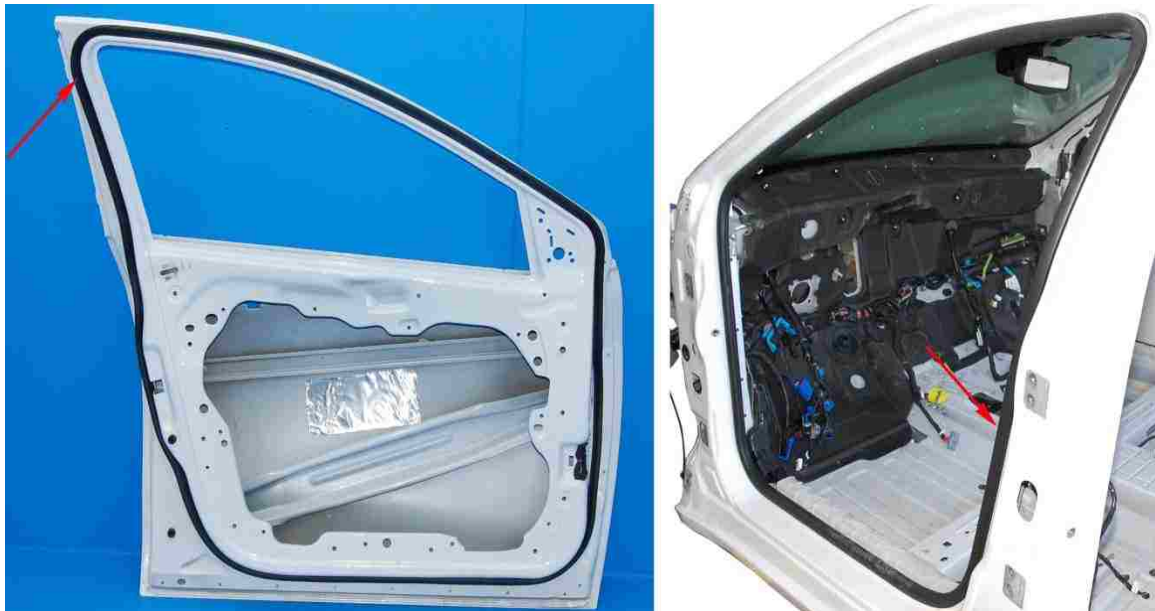
Figure 1-2: Weatherstrip seal system on door frame and car body [1]. The sealing system includes both the seals on the door and the ones applied to the vehicle body where the door fits when closed.
