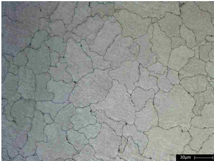
Figure 4- 21. Optical micrograph showing grain structure of CaC_2 -treated AM60 in a cylindrical coupon in T4 condition.
