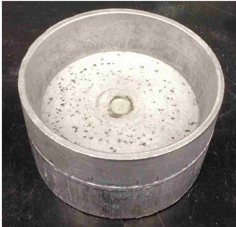
Figure 4- 1. Squeeze cast cylindrical coupon.
