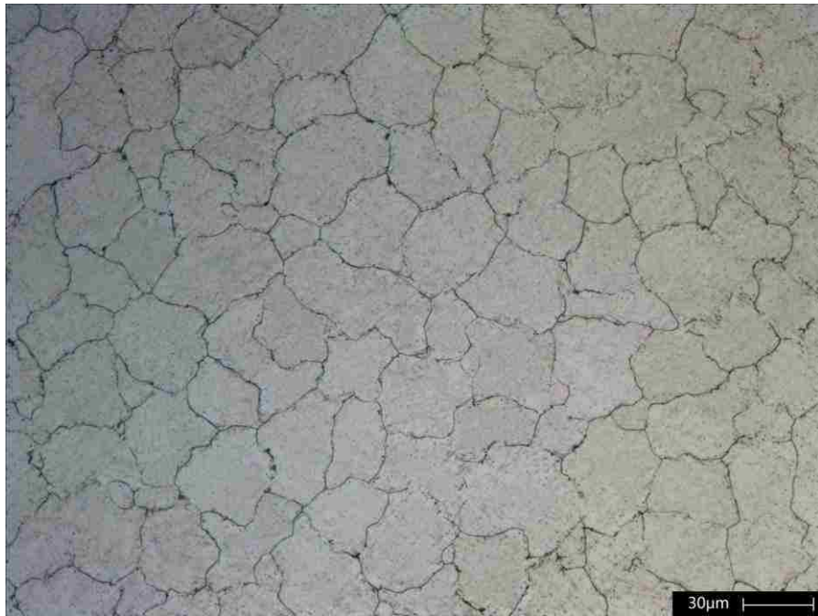
Figure 4- 20. Optical micrograph showing grain structure of C_2Cl_6 -treated AM60 in a cylindrical coupon in T4 condition.
