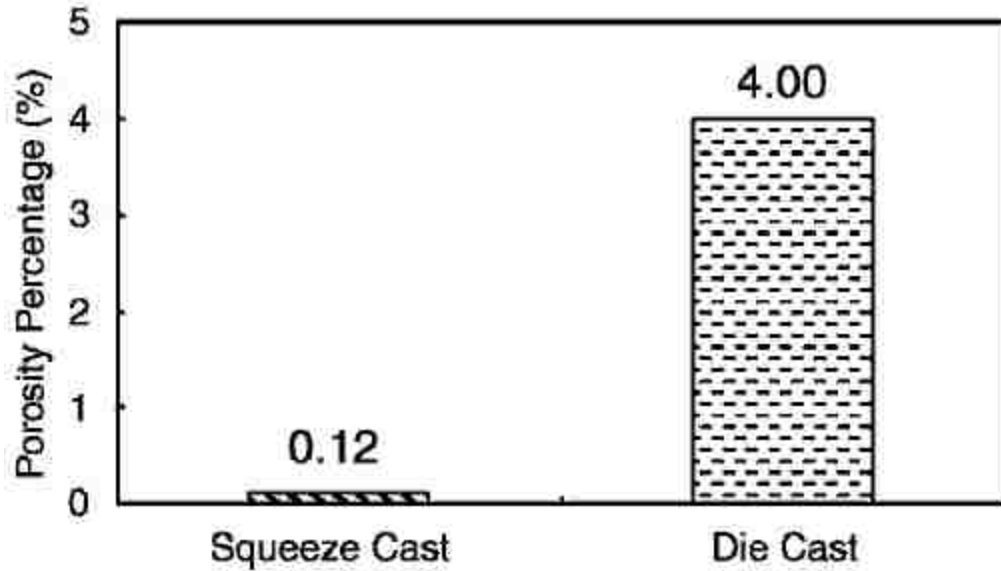
Figure 2- 8. Porosity levels of squeeze cast and die cast AM50 alloy [28].
