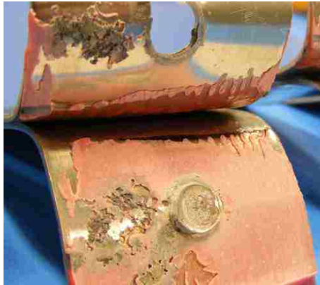
Figure 4-20. RSW and Dow coach joint 1.3 mm showing adhesive failure.
