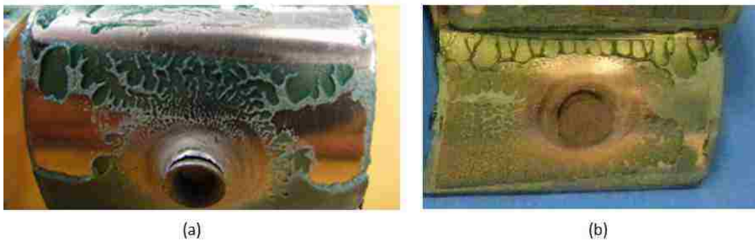
Figure 4-29. Adhesive layer failure mode analysis, SPR + Sika coach joint (a) 1.3 mm , (b) 1.75 mm.
