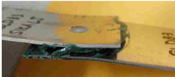
Figure 4-31. Lap Joint RSW + Sika; the test was stopped after the adhesive layer failure and before the nugget failure.
