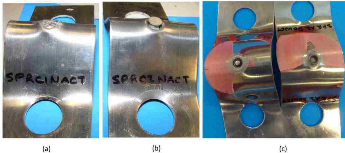
Figure 4-67. Failure mode Cross Tension SPR joints. (a) Rivet tail pulled out from the bottom sheet. (b) Rivet head pulled out the top sheet; rivet still stuck in the bottom sheet. (c) Adhesive failure of the adhesive layer.
