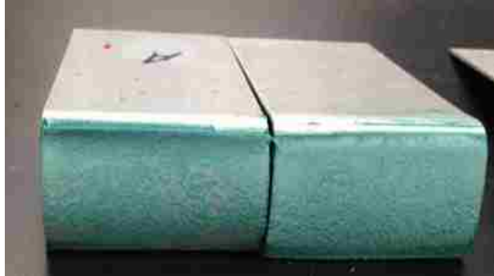
Figure 4-30. Adhesively bonded coach joint prepared in “ideal conditions”; prepared by SIKA engineers.
