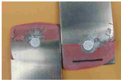
Figure 4-41. Adhesive layer failure mode, 1.75 mm Lap Joints RSW + Dow.
