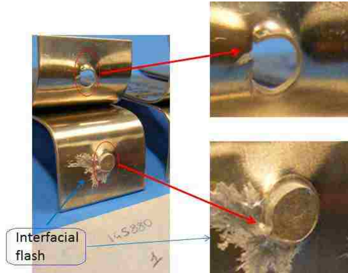
Figure 4-17. Failure mode analysis of RSW coach joints; highlighted in red the lip on the nugget and the corresponding tearing of the material on the opposite sheet and in blue the interfacial flash (weld expulsion).
