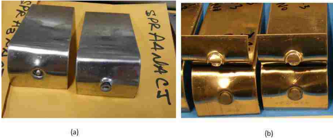
Figure 4-28. Rivet failure mode analysis, (a) rivet tail pull-out. (b) rivet head pull-out.
