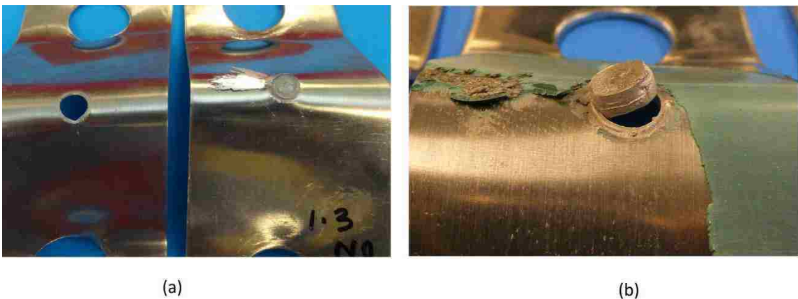
Figure 4-59. RSW cross tension joints failure mode. (a) nugget pull-out; (b) tilting of the nugget induced by the asymmetric loading conditions.
