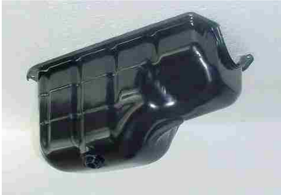
Figure 2.7-1: Oil pan in steel sheet of FIAT 8V Fire engine [8].
