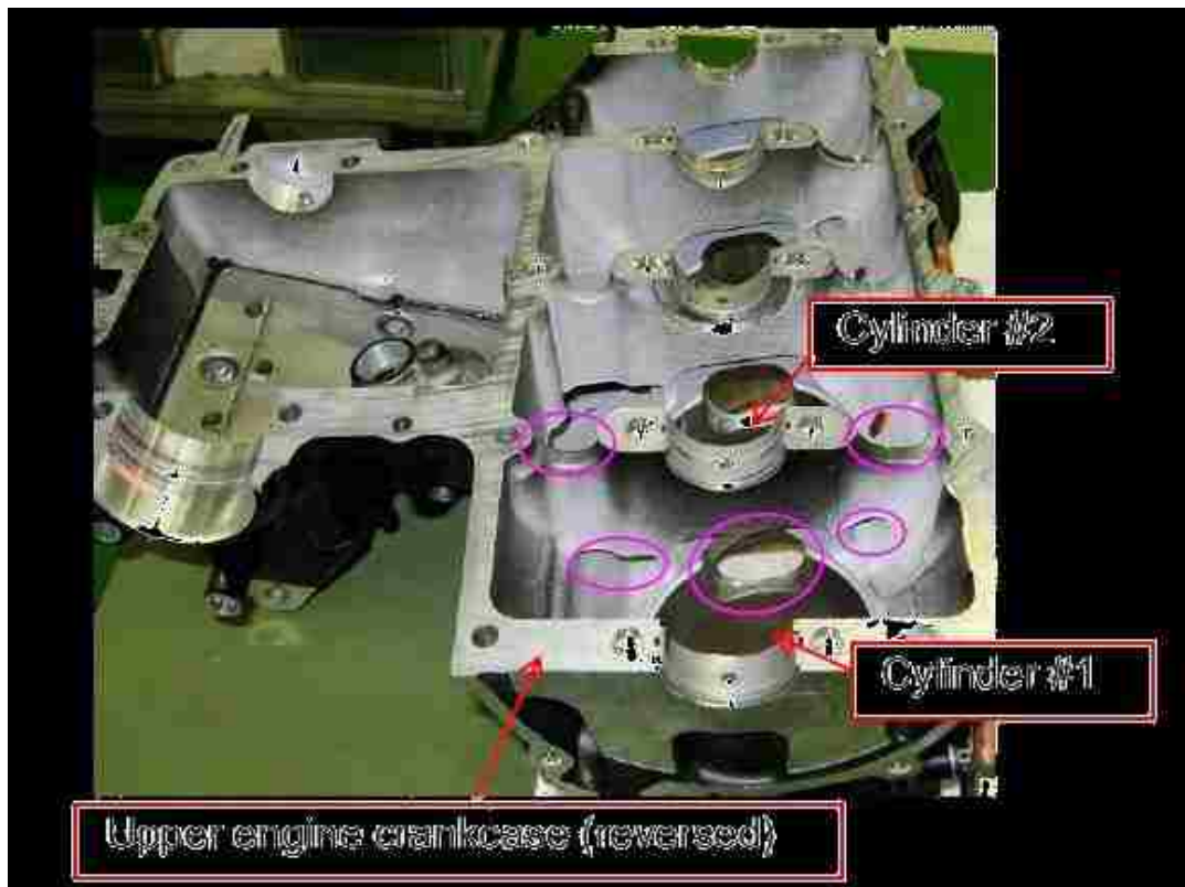
Figure 3.4-1: Breather (or breathing) holes between cylinder 1 and cylinder 2 [30].
