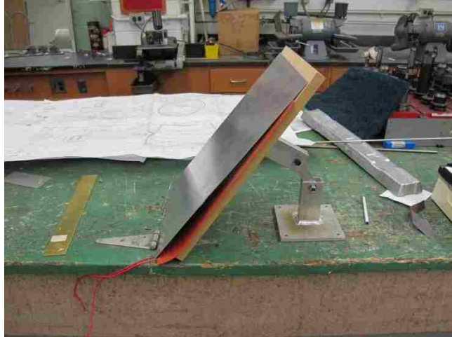
Figure 3.9: Inclining base where flat plate is installed.
