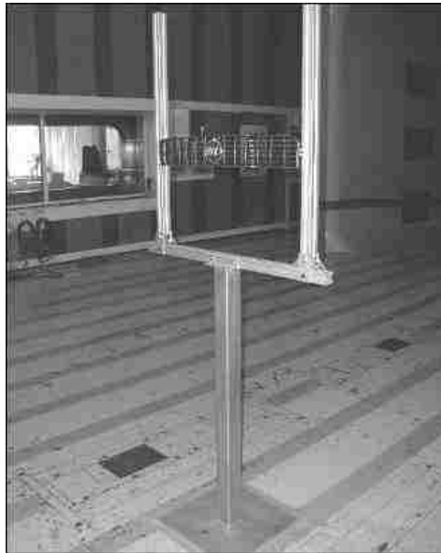
Figure 7: Experimental Setup for Flow Test on Isolated Front Grill Component
