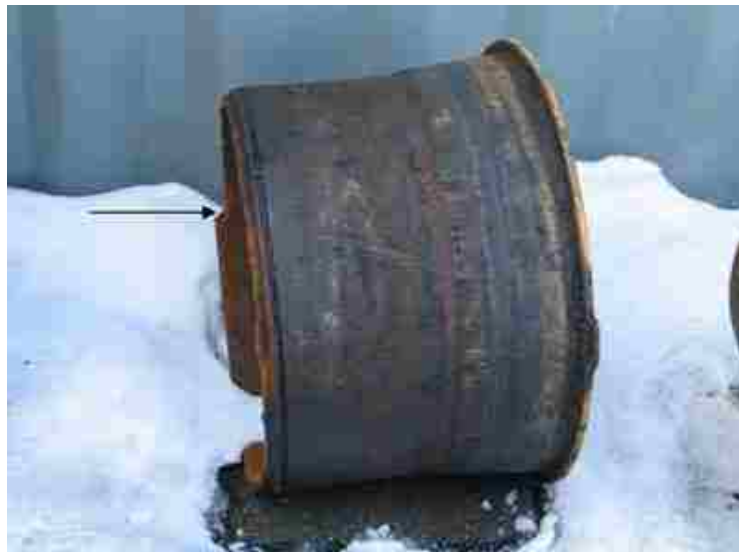
Figure 2.1: 2007, Massachusetts, USA wheel failure. Black arrow indicates failure region [4].
