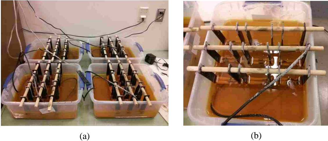
Figure 3.1: Accelerated corrosion test setup: (a) all corrosion containers, and (b) top view of one corrosion container
