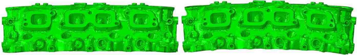
Figure 65: Head Deformation for Cold Clamping (left) and hot Clamping (right) at 100X, No Section
