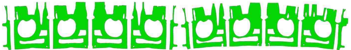
Figure 68: Deformation for Cold Clamping (left) and hot Clamping (right) at 100X, Section cut at Long Length Studs
