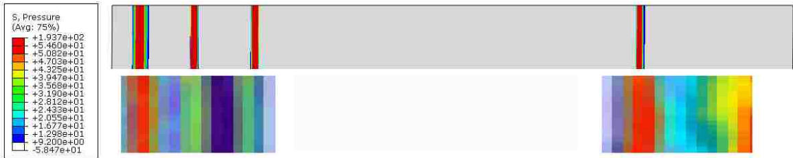
Figure 39: Comparison of 180° Section (top) with Fuji Film (bottom)
