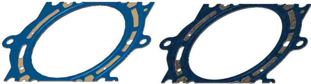
Figure 24: Surface model of the gasket assembly (Left) and meshed shells of gasket assembly (right)
