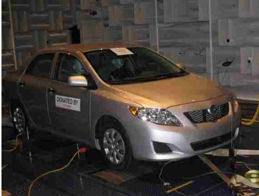
Figure 3: Vehicle in a semi-anechoic dynamometer for speech, impulse response and background noise measurements with example HATS units' configuration; B&K Type 4100 HATS in the driver location as the receiver, or the listener, and B&K Type 4128 HATS in the passenger front location, as the source, or the talker.
