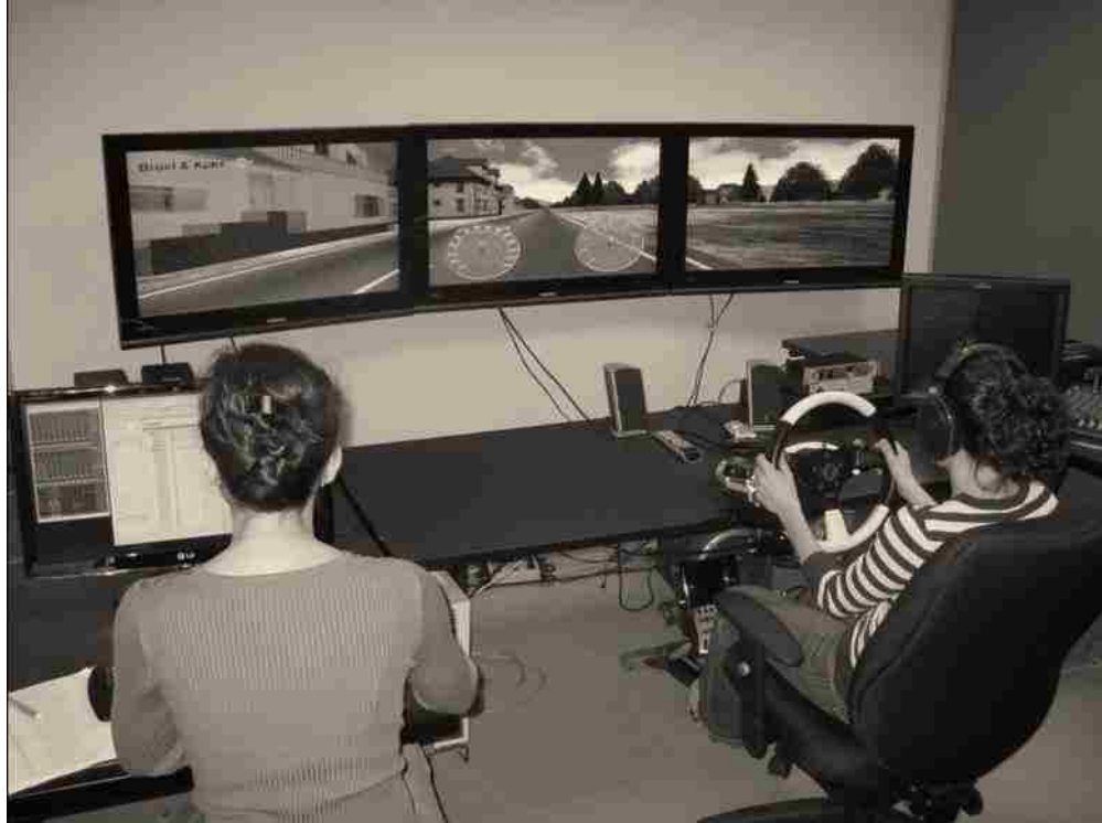
Figure 6: A juror (right) driving the NVH Simulator while the HINT sentence recordings are delivered from the NVH Simulator software (left). The levels of the consecutive HINT sentences are adjusted in 2 dB increments, based on the juror's response.
