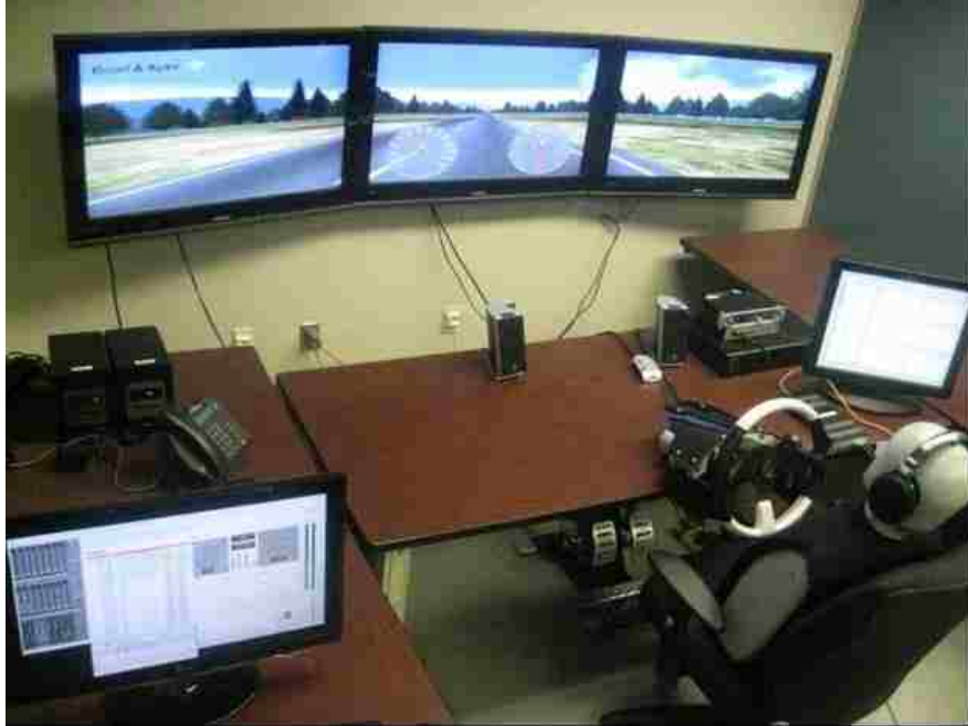
Figure 5: The sound pressure levels associated with the HINT sentences to be delivered from the NVH Simulator software through the headphones matched those recorded inside the vehicle to within 0.2 dB, in the range from about 45 dBA to 70 dBA, in increments of 2 dB. The headphones were placed on a Type 4100 HATS and the levels were verified using the PULSE LabShop software version 16. The HINT calibration signal recorded at these levels and different configurations inside the vehicle was used as a benchmark for any needed adjustments using the NVH Simulator software and the NVH Simulator soundcard mixer.
