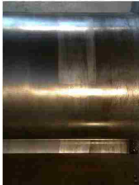
Figure 10. Image showing material transferred from the stock surface to the work roll surface after the two-pass rolling on the Robertson mill [15]
