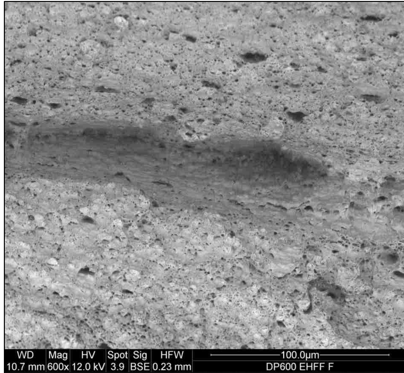
Figure 5.17: Backscatter image of a crack in EHFF specimen
