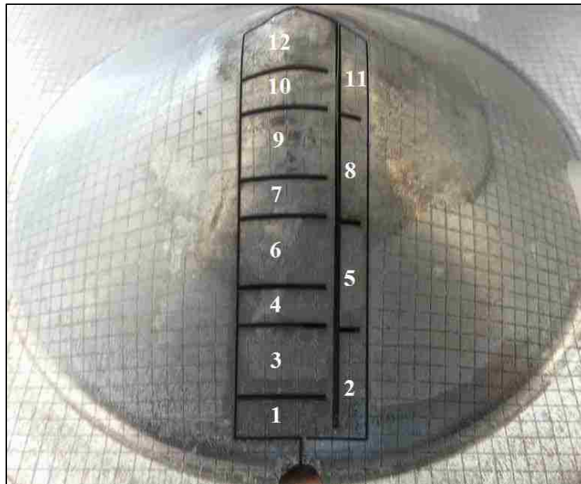
Figure 3.8: EHDF specimen cut using EDM. Samples: 1, 4, 7, 10 - Longitudinal; 2, 5, 8, 11 – Transverse; 3, 6, 9, 12 – Plan.
