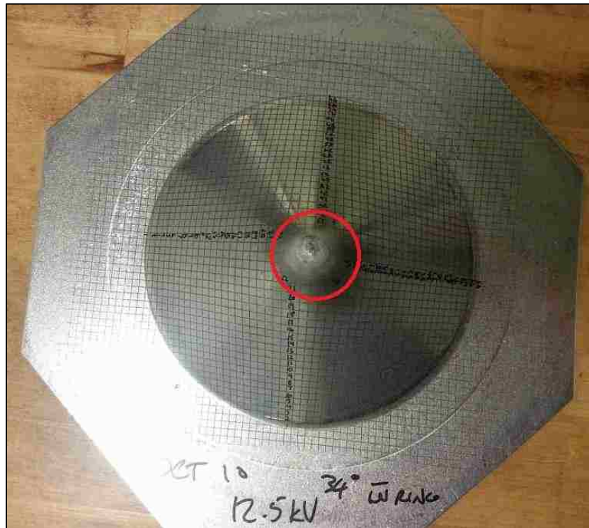
Figure 3.7: Severe surface damage to the apex of EHDF sample preventing grid analysis
