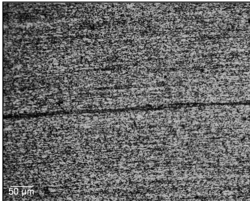
Figure 5.1: Martensite banding in DP600
