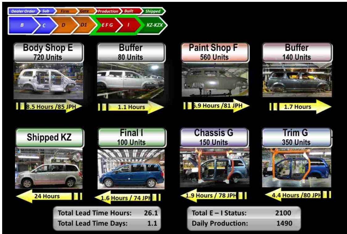
FIGURE 3- 1 THE VEHICLE ASSEMBLY PROCESS AND LEAD TIME IN PLANT
