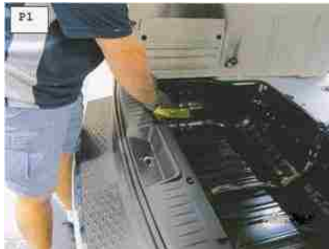
FIGURE 3- 2 REMOVE THE REAR SCUFF PLATE
