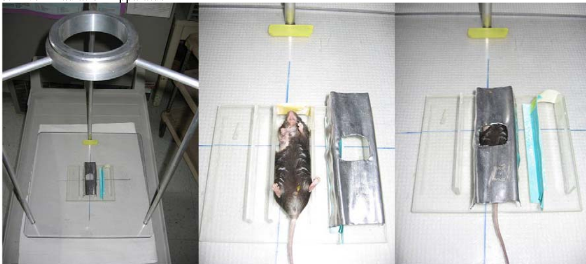
Figure 1. a. A flowchart of the experiment design. b. Liver specific irradiation apparatus. The radiation source was placed in the ring at the top. The mouse was anesthetized and placed in a holding box. A lead shield limited irradiation to the upper abdomen.
