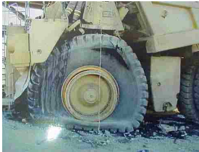
Figure 2.3.1 – Result of tire zipper failure [21].
