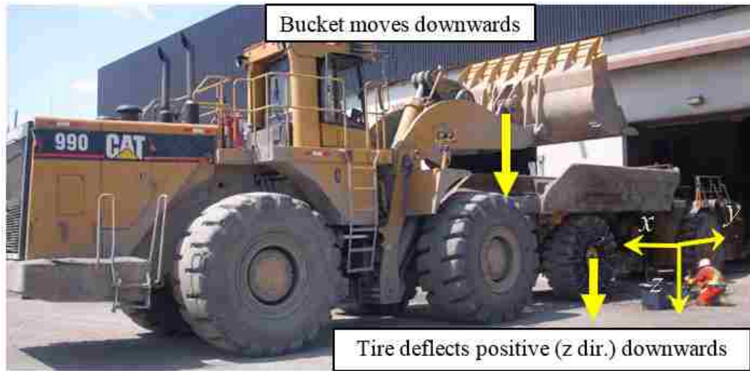
Figure 4.3.1 - Excitation of the AD45B test vehicle using the Caterpillar 990 front load scoop.
