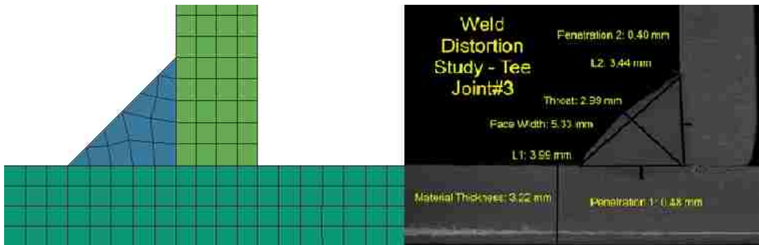
Figure 4.3- Software section (left) and real section (right) of the T-joint for transient analysis
