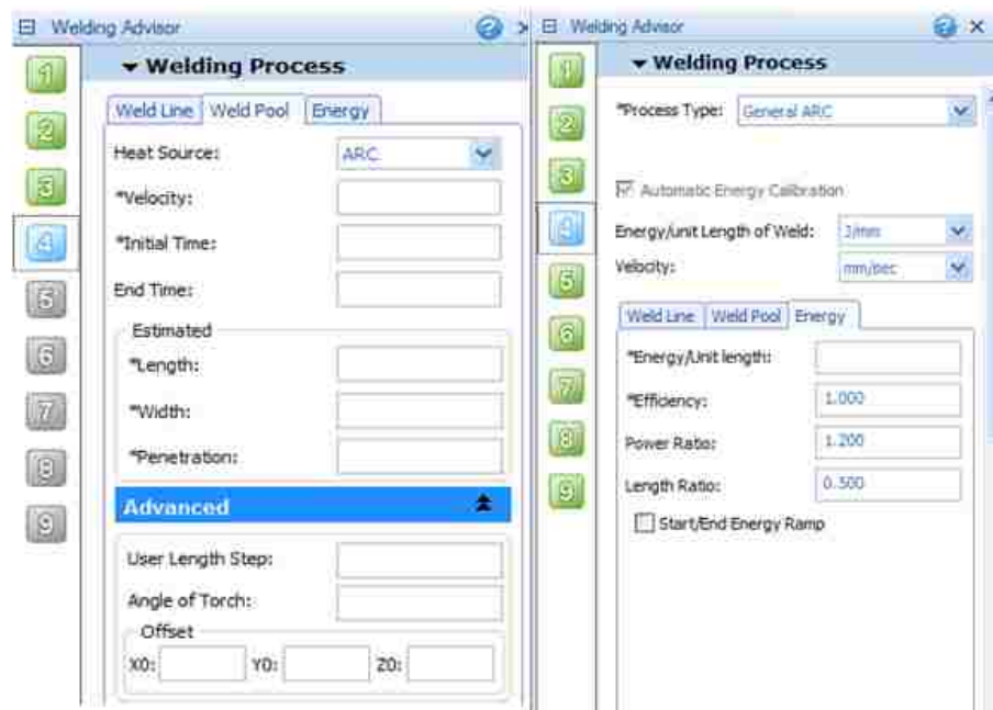
Figure 8.5-Parameters require for the welding process (Step 4)
