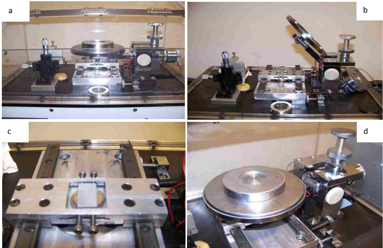
Fig. 3.1 Sliding tribotester attached on (a) Sciland Pin/Disc Tribometer PCD-300A (b) load cell and cantilever beam, (c) sample holder for reciprocating mode (d) sample holder plus load
