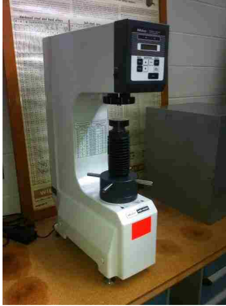
Figure 4.4: Mitutoyo HR 400 Rockwell hardness testing machine used during the project.
