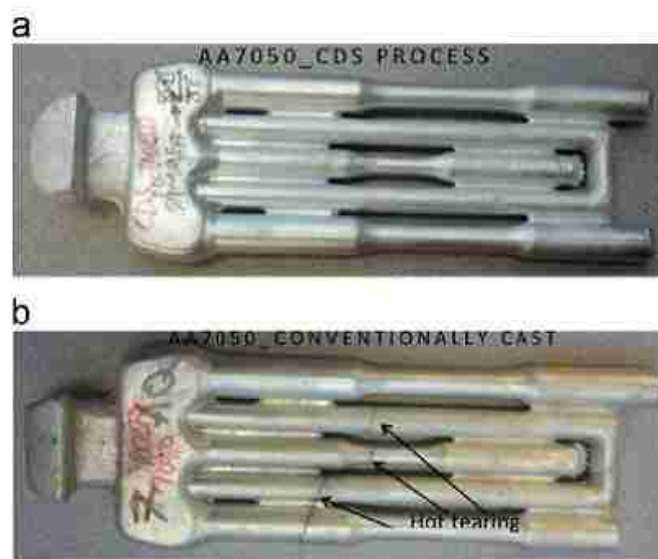
Figure 3.1: Differences between samples cast with the CDS process (a) and a conventional casting technique (b) [9].
