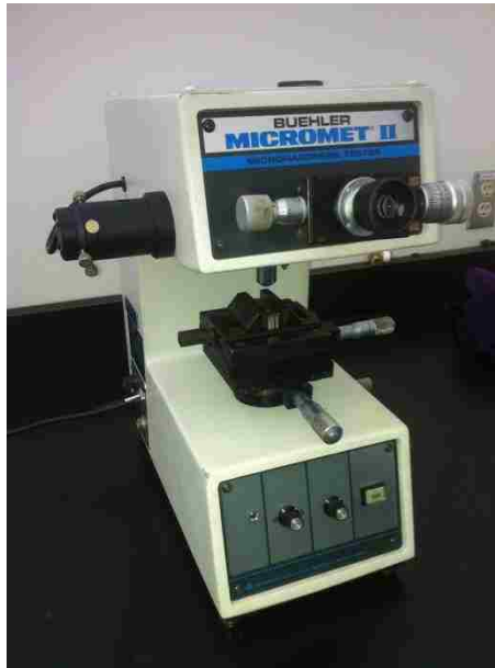
Figure 4.6: Buehler Micromet II microhardness testing machine used during the project.
