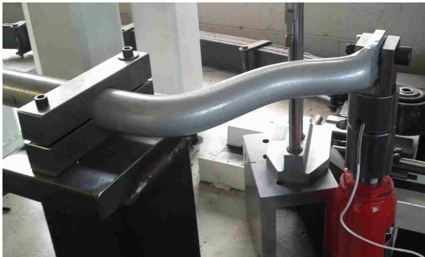
Figure 5.8: Physical testing setup: actuated end with steel bushing
