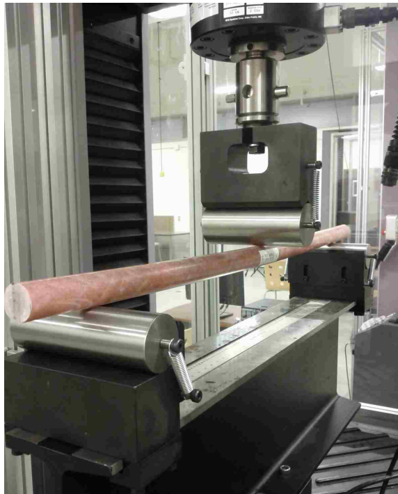
Figure 4.7: Experimental setup: three point flexure test (sample 1C)
