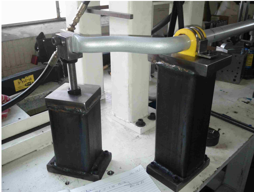
Figure 5.7: Physical testing setup: fixed end with polymer bushing
