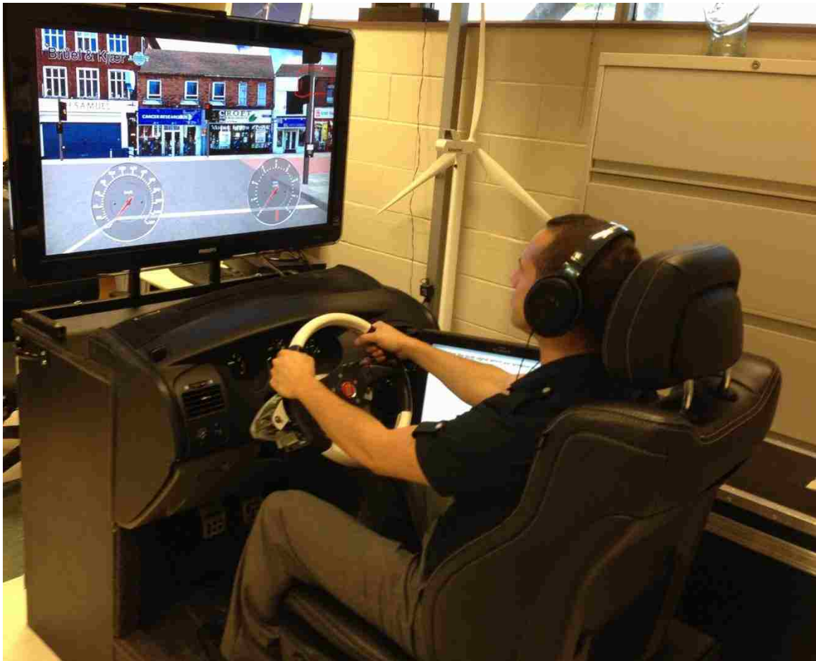
Figure 20: Juror in the NVH driving simulator buck participating in evaluation
