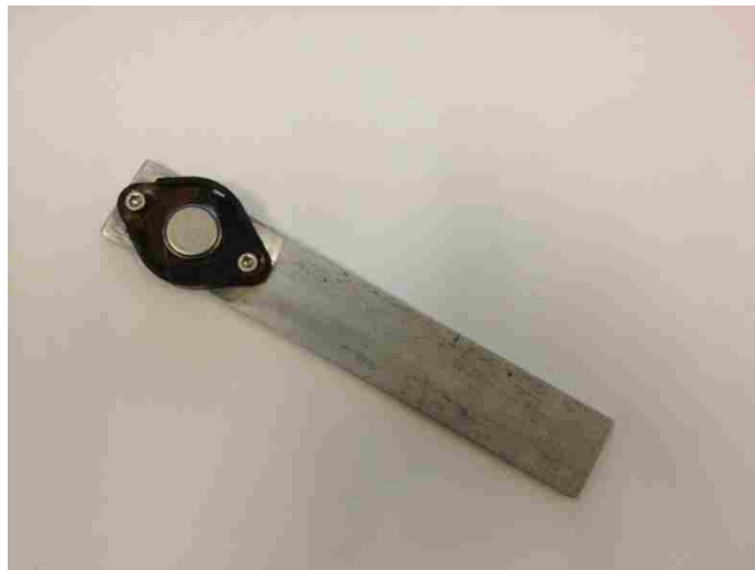
Figure 5: An iButton sensor fixed on an aluminum plate
