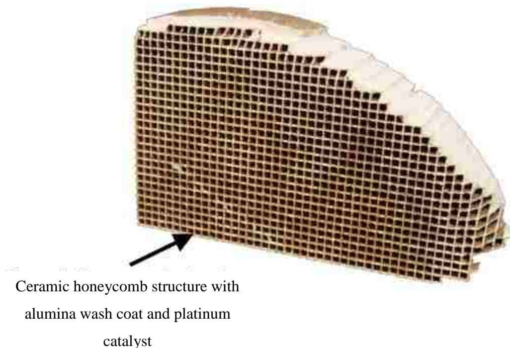
Figure 1.4. Diesel oxidation catalyst – cutaway section
