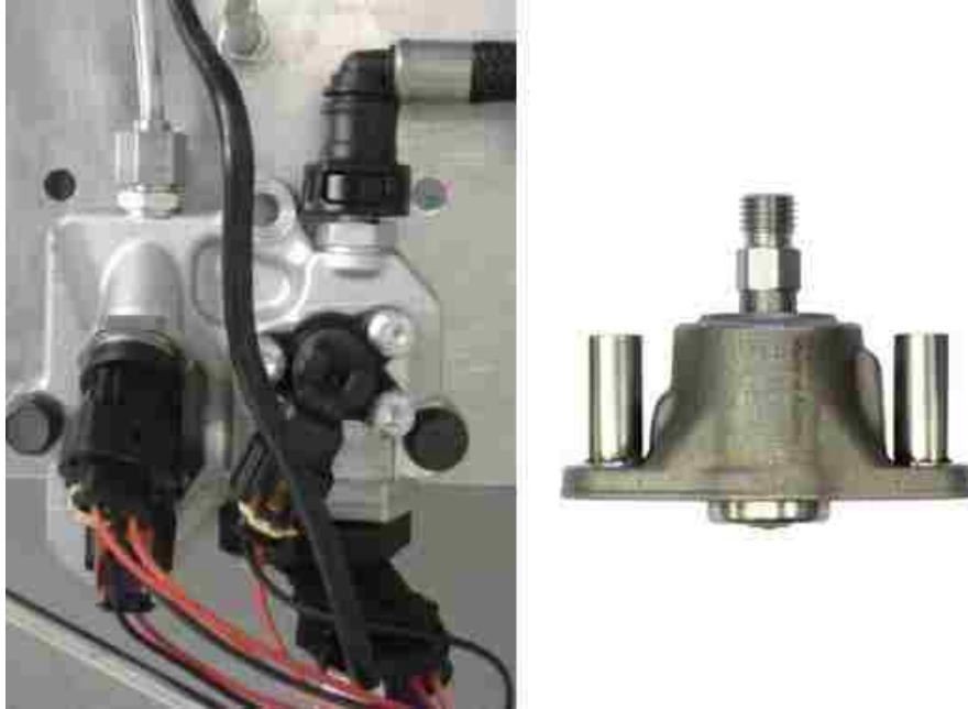
Figure 4.3. Bosch Departronic System (Left: Shut-off and doser valve, Right: Injector)
