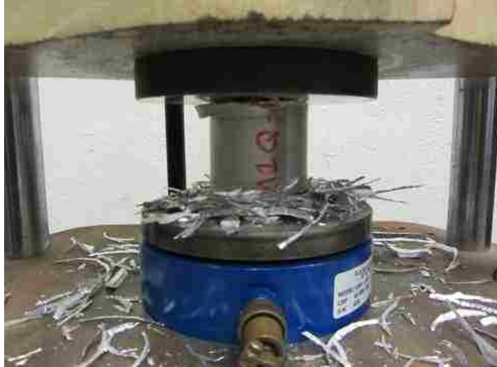
Figure 2.3 Shards produced by an AZ31B Mg extrusion 3.175 mm thick and 65 mm outer diameter subjected to quasi-static axial crushing [16].
