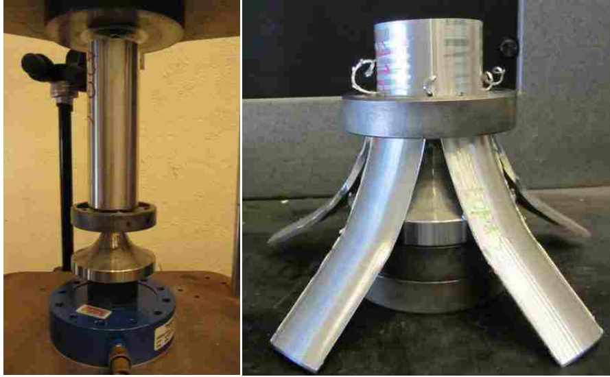
Figure 2.10 Experimental setup of AA6061-T6 extrusion in quasi-static cutting before test (left) and after test (right) using 5 blades.
