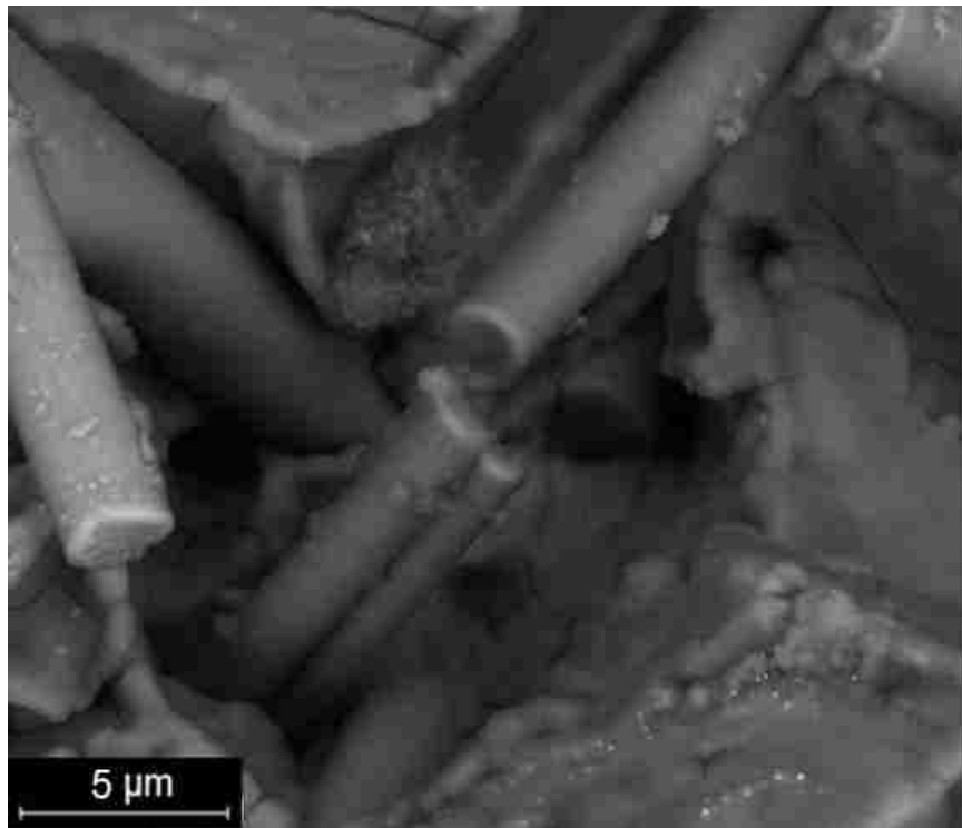
Figure B.16. High magnification fracture of AM60-based composite with 5 vol% Al 2 O 3 fibre + 3 vol% nano Al 2 O 3 particle
