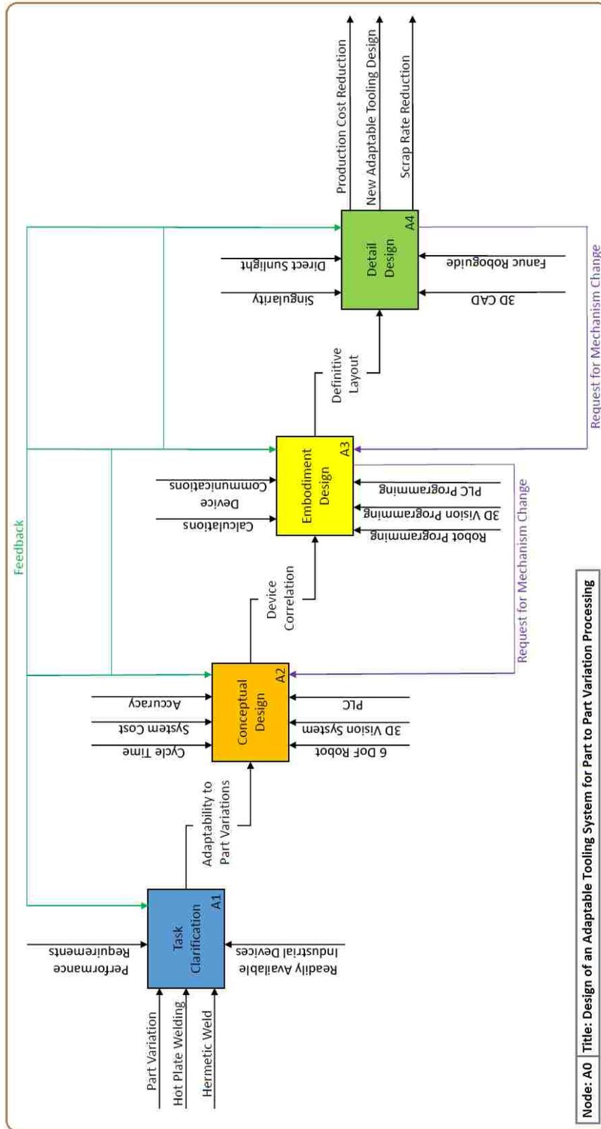
Figure 32-Decoupled Node A0
