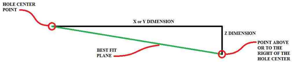
Figure 62-X and Y Minor Plane Calculation © 2017 IEEE
