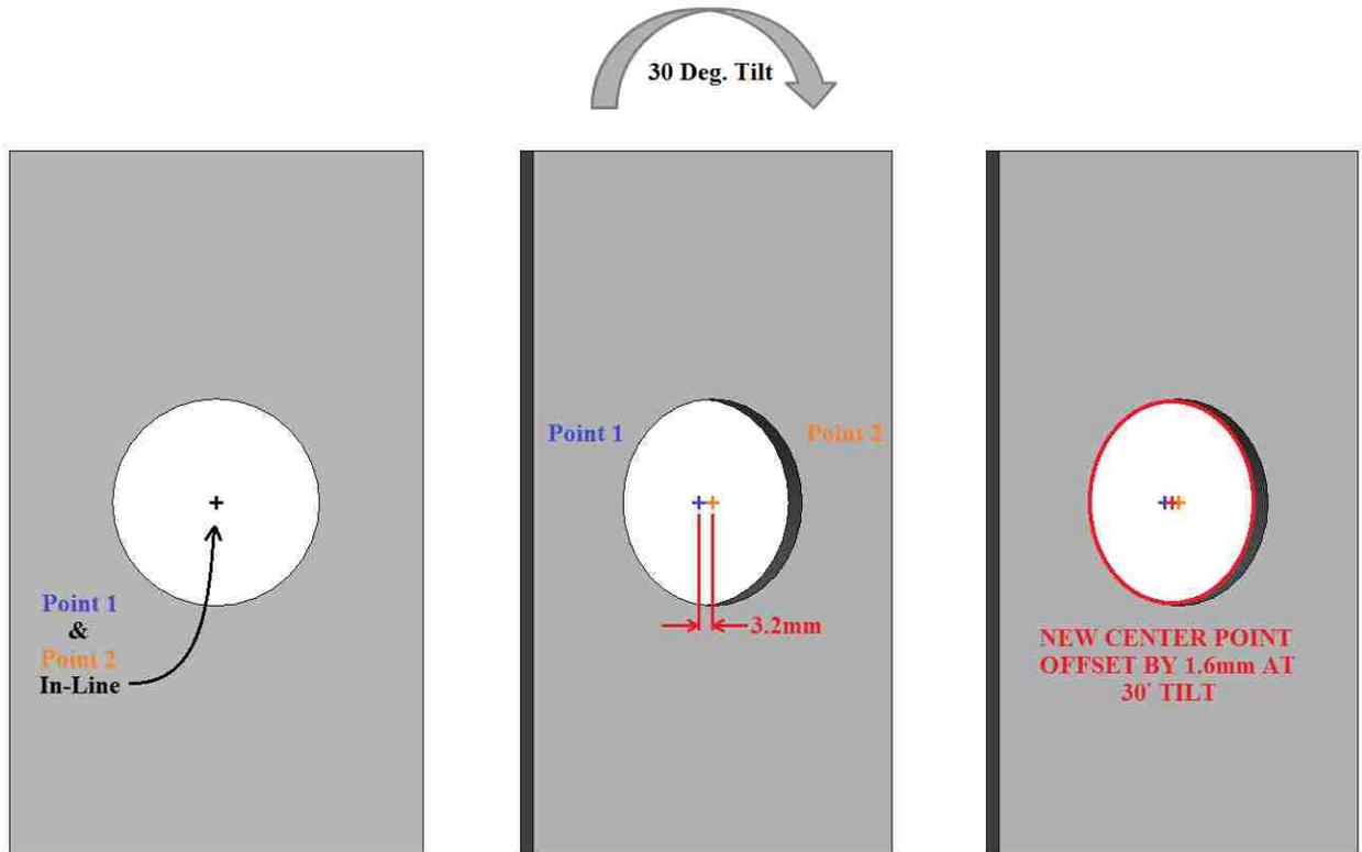
Figure 78-Object Tilt Illustrating Hole Offset in 3D CAD
