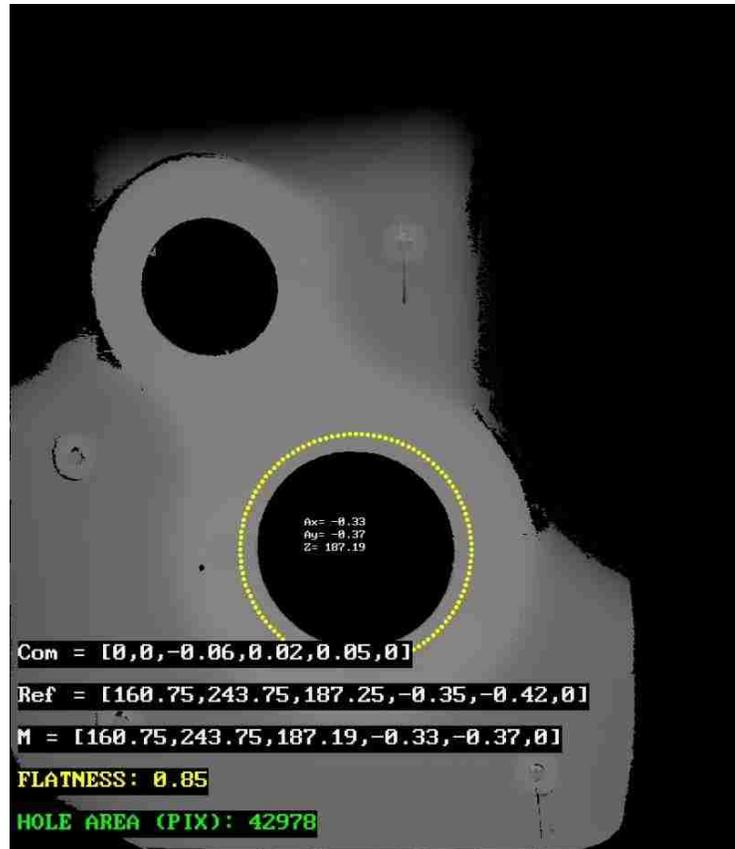
Figure 73-Image Scan Repeatability Test
