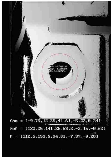
Figure 77-Scan Affected by Direct Sun Light Exposure
