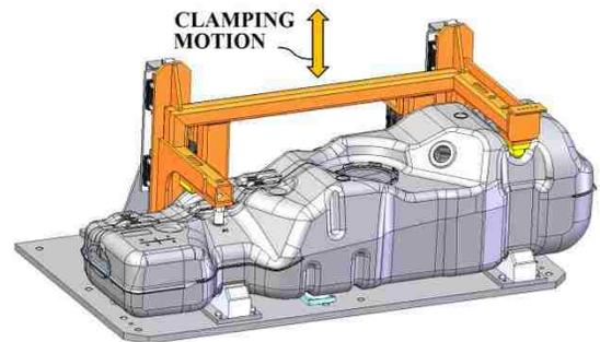
Figure 8-Fuel Tank Clamping (Courtesy SPM Automation (Canada) Inc.)
