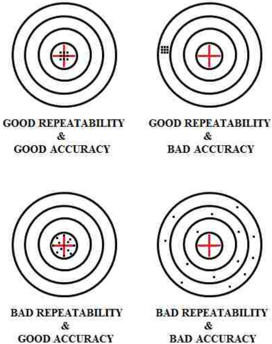
Figure 65-Robotic Accuracy and Repeatability Illustration
