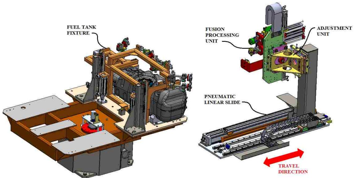
Figure 4-Fixed Mounted Fusion Unit Position Relative to the Fuel Tank Fixture
