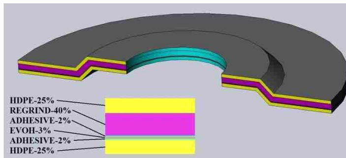
Figure 13-Fuel Tank Blow Moulding Layers
