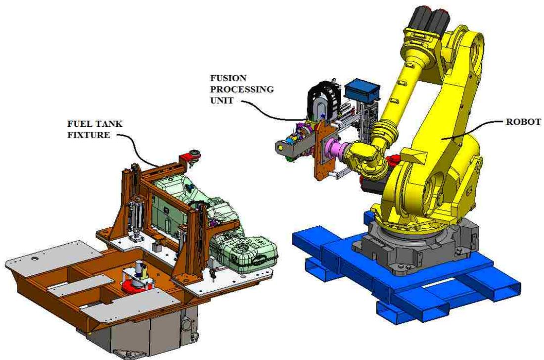
Figure 5-Robot Mounted Fusion Unit Position Relative to the Fuel Tank Fixture
