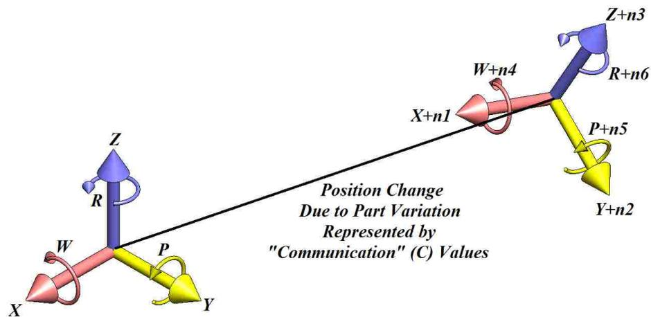
Figure 26-Robot Position Change
