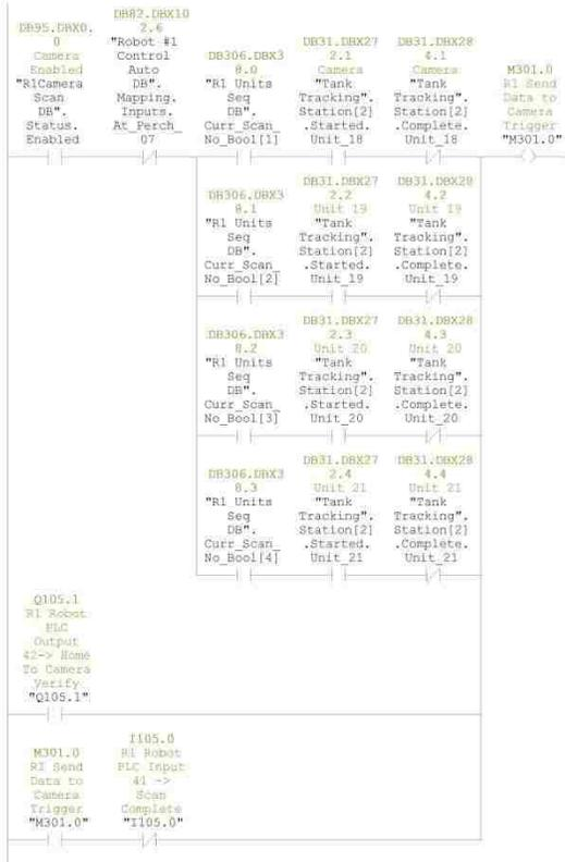
Network: 11 Generate the rising edge SEND\_REQ to start the T\_SEND function
