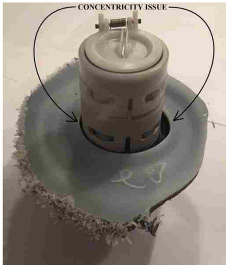
Figure 11-Part Welded Out of Concentricity
