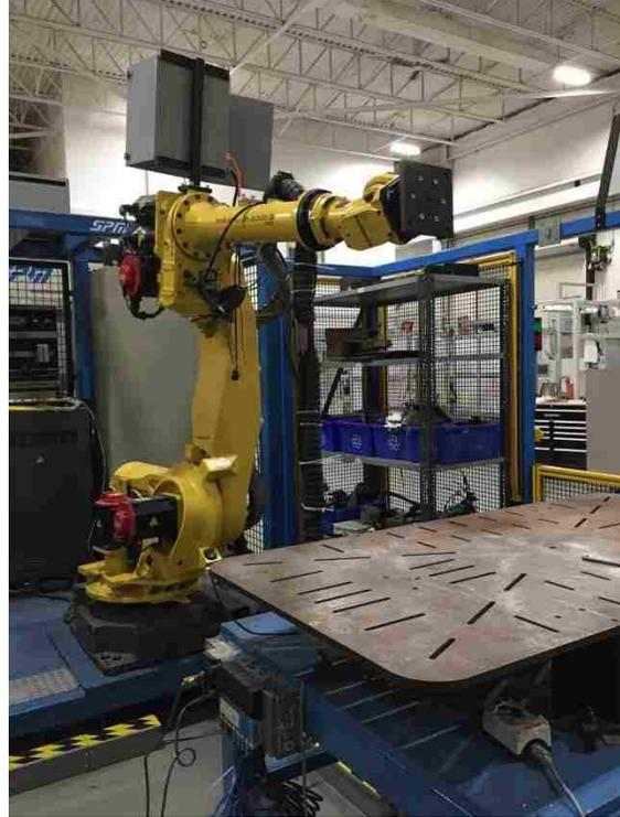
Figure 37-Test Robot-Fanuc R2000 iB 165F
