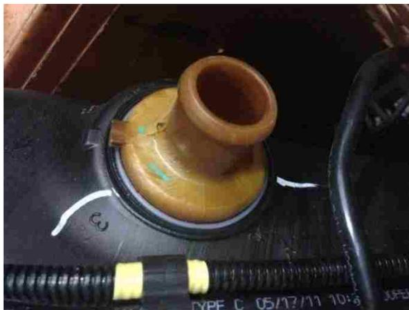
Figure 1-Inlet Check Valve
