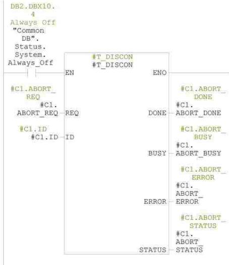
Network: 17 Generate the raising edge for T\_DISC function block
