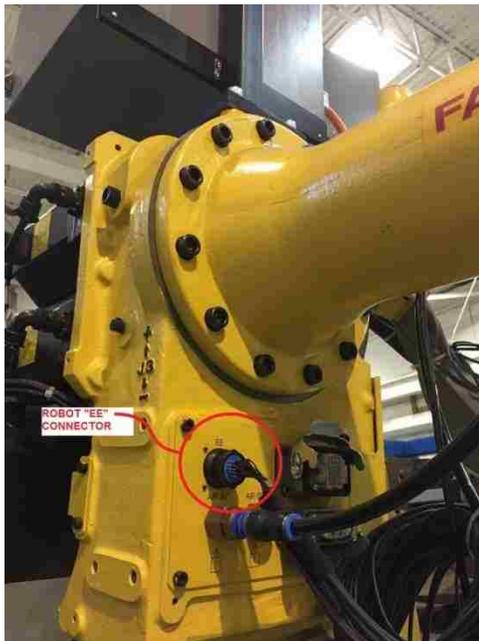
Figure 45-Robot EE Connector
