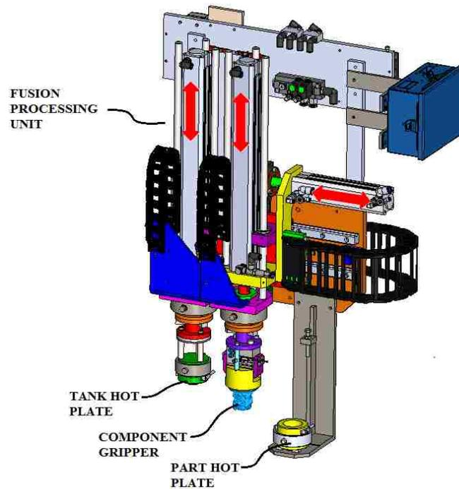
Figure 19-Fusion Unit Design (Courtesy SPM Automation (Canada) Inc.)
