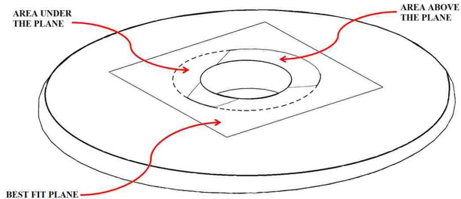
Figure 59-Best Fit Plane Placement on 3D Surface © 2017 IEEE
