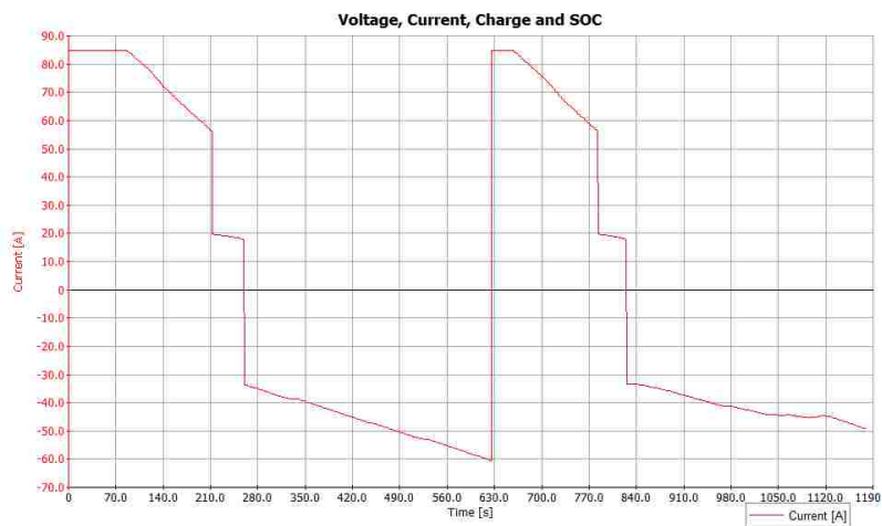
Figure 8.6 Dynamic battery charge and discharge
