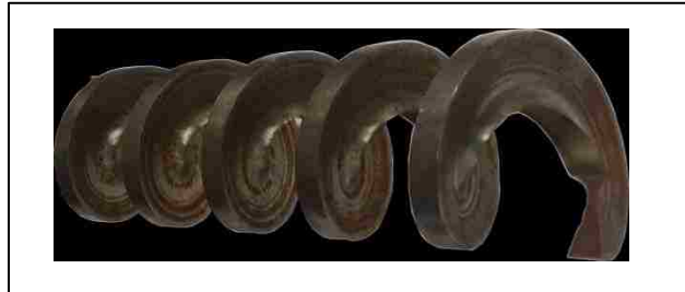
Figure 5-7: Helical Insert after Manufacturing
