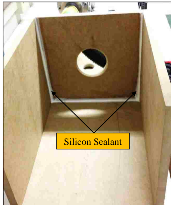
Figure B-1: Sealing of Air Box Joints
