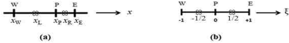
Figure 4.4 Stencil with five discretisation points for the 4 th -order scheme
