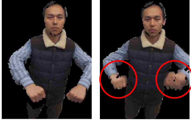
Figure 7.3: Frames with large motion blur (right image) might be selected if \{c_m^t(k)\} in Equation 7.6 is excluded.
