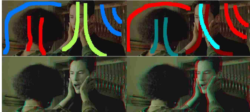
Figure 5.10: The scene of stationary camera and static objects will fail the three algorithms in the preprocessing. However, the two labeling brushes: depth difference brush and depth equivalence brush can still produce similar visual 3D effect as does Guttman's method. Guttman's method (left column) assigns different depth (color coded) to different layers of the scene. My method (right column) achieves the same effect by applying the depth difference brush twice. The dark red&cyan scribbling pair indicate the depth difference of the old lady and the young man. And the light red&cyan pair point out the difference between the young man and the background. The results from both methods are visually comparable.
