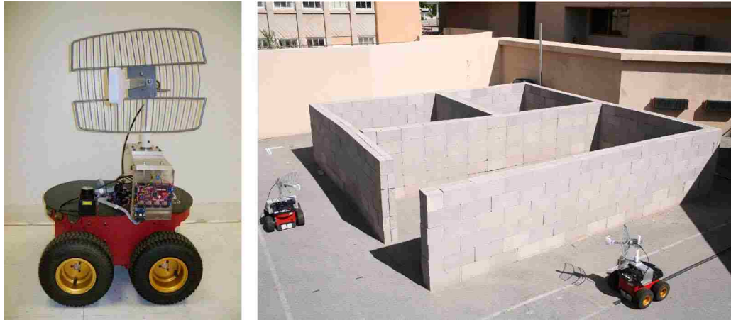
Figure 5.14: (left) A Pioneer P3-AT robot equipped with our servo control mechanism /fixture, adaptive narrow-beam directional antenna and Hokuyo laser scanner; (right) two robots using laser scanners and wireless measurements in order to map an obstacle structure that includes occluded parts.
