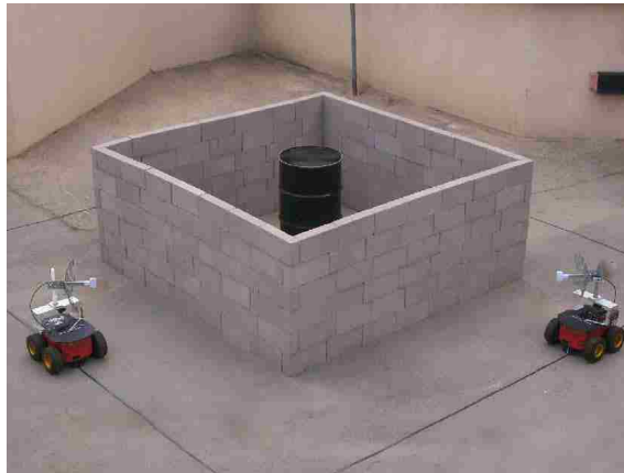
Figure 4.6: (left) Two pioneer 3-AT robots equipped with our servo control mechanism/fixture and an adaptive narrow-beam directional antenna in action, making wireless measurements in order to map the obstacle.
