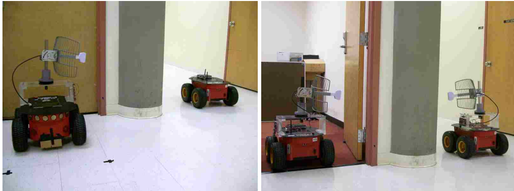
Figure 2.12: (left) Pioneer robots gathering data at the basement of our building with the transmitter using an omnidirectional antenna and the receiver using a directional one. (right) Pioneer robots using directional antennas for both transmission and reception.
