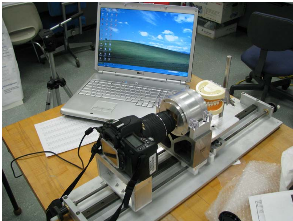
Figure 4.7 Overview of the multi-view imaging system.
