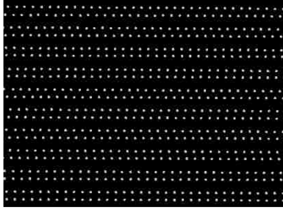
Figure 2.4: Irregular spacing of LiDAR data points
