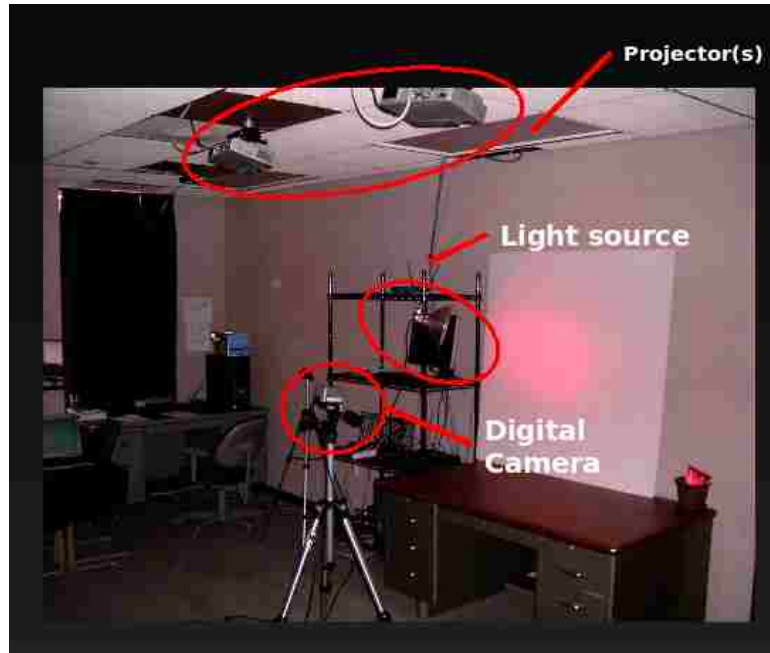
Figure 4.1: A projector-camera system equipped for image display as well as focused-light and ambient-light aberrations.
