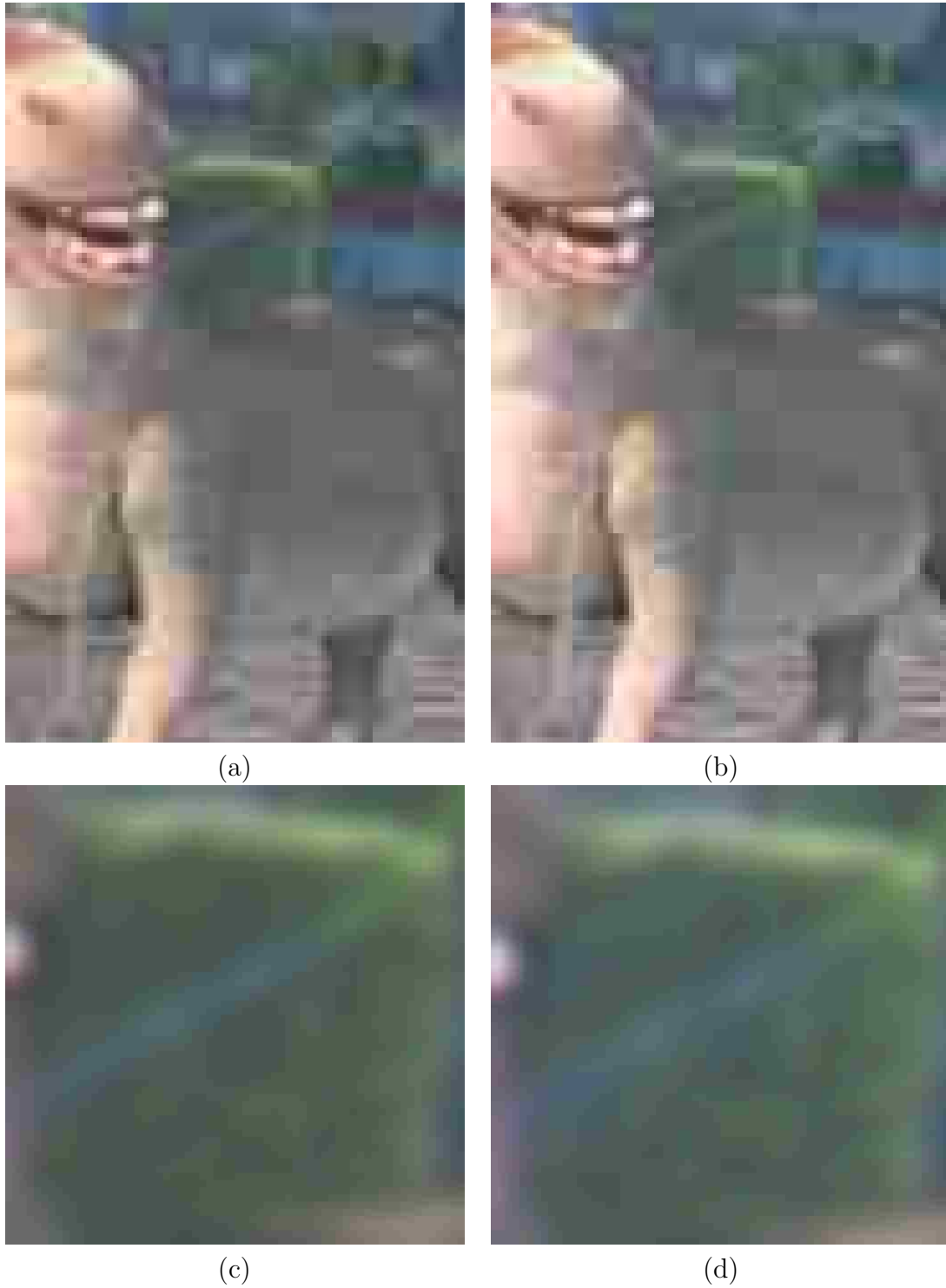
Figure 4.3: Uncorrected and corrected camera images with close-up of aberration portion. (a)The aberrated/ uncorrected version of the input image. (b) The aberrated/ corrected version of the input image. (c) Blue portion of aberration region of uncorrected image magnified. (d) Blue portion of aberration region of corrected image magnified.
