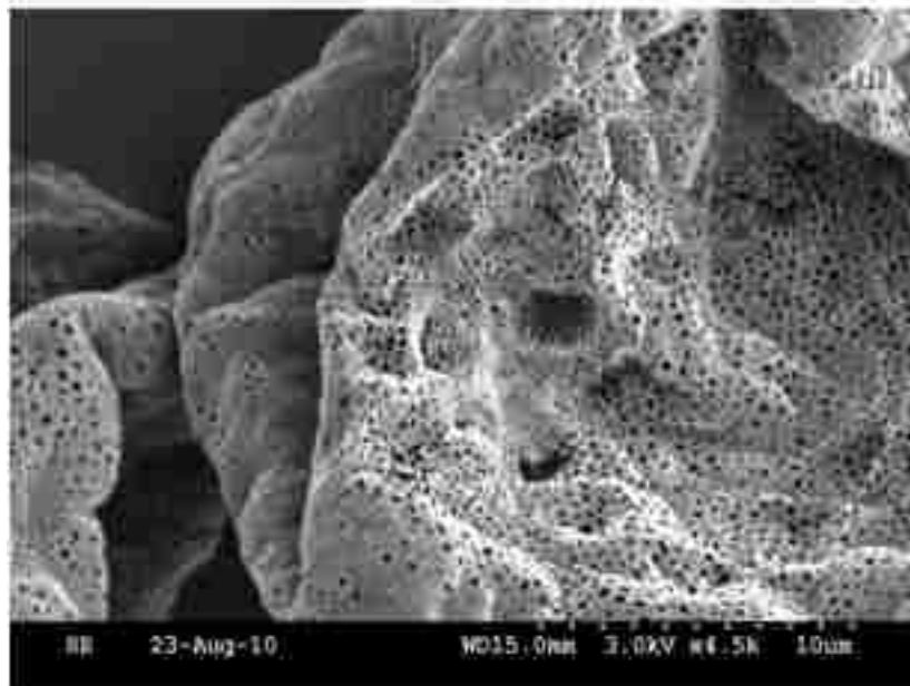
Figure 4.2: Effect of higher evaporation rate on particle morphology; Particles of PS-PMMA obtained from a 2wt% polymer solution in DCM using a 15 \mu\text{m} orifice (a) collapsed particles with large surface indentations. (b) surface perforations on the particles due to rapid evaporation of DCM.
