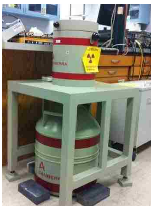
Figure 6: Germanium detector at Washington University School of Medicine
